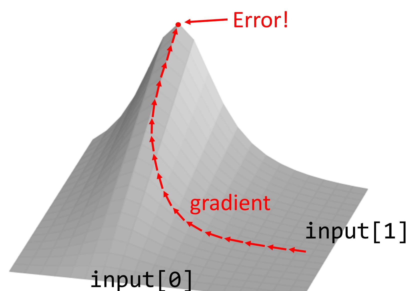
Gradient can be used to guide searches over large input spaces.
