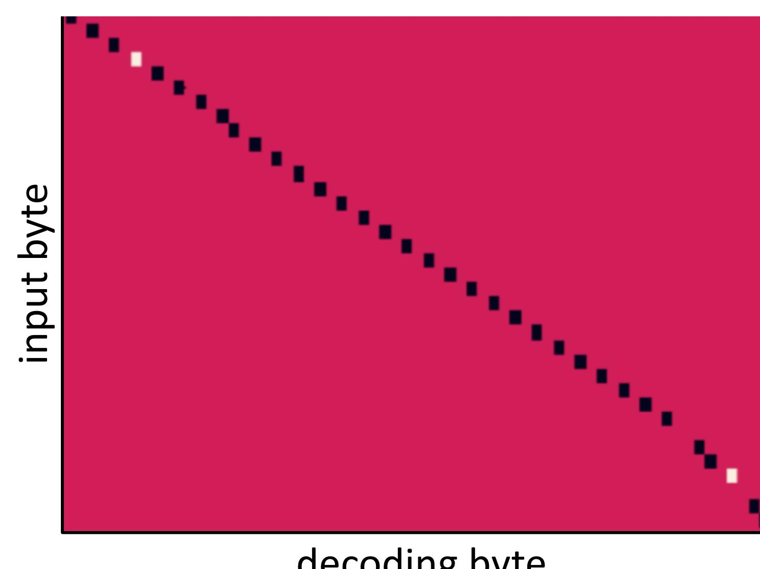
Gradient Analysis identifies which input bytes are used to look up each Huffman decoding index in gzip decompression.
